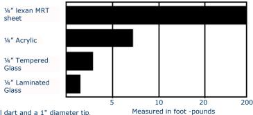
1 ) Drop Dart Test with a 5-lb steel dart and a 1" diameter tip.
